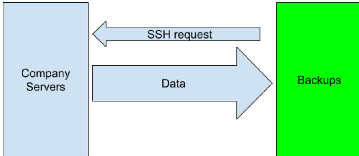
The problem here is that a compromised backup server can access its clients, and compromise them as well. Additionally, there is no way for the backup server to detect whether the data on the main server has been tampered with, so if there is an attack and the data is pulled on schedule, it can still damage the backups.
