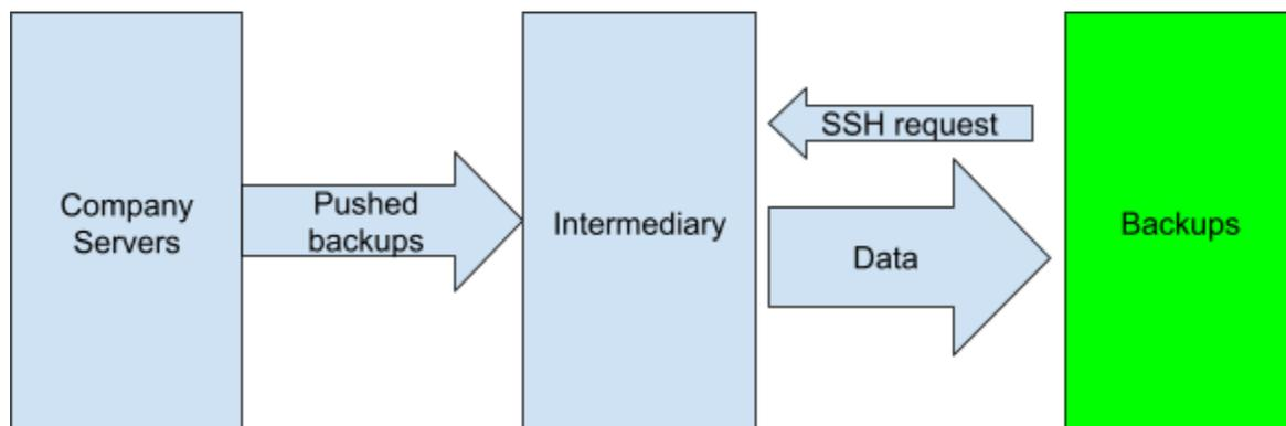
In this case, no connection is ever established between the backup server and the company servers, so they are isolated from one another, and any infection is contained.
